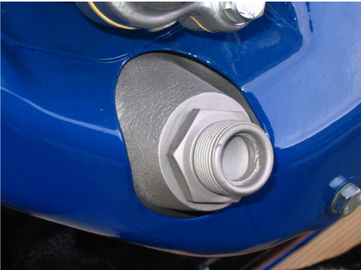
Figure 2. EGR port on exhaust manifold plugged with expansion plug.
