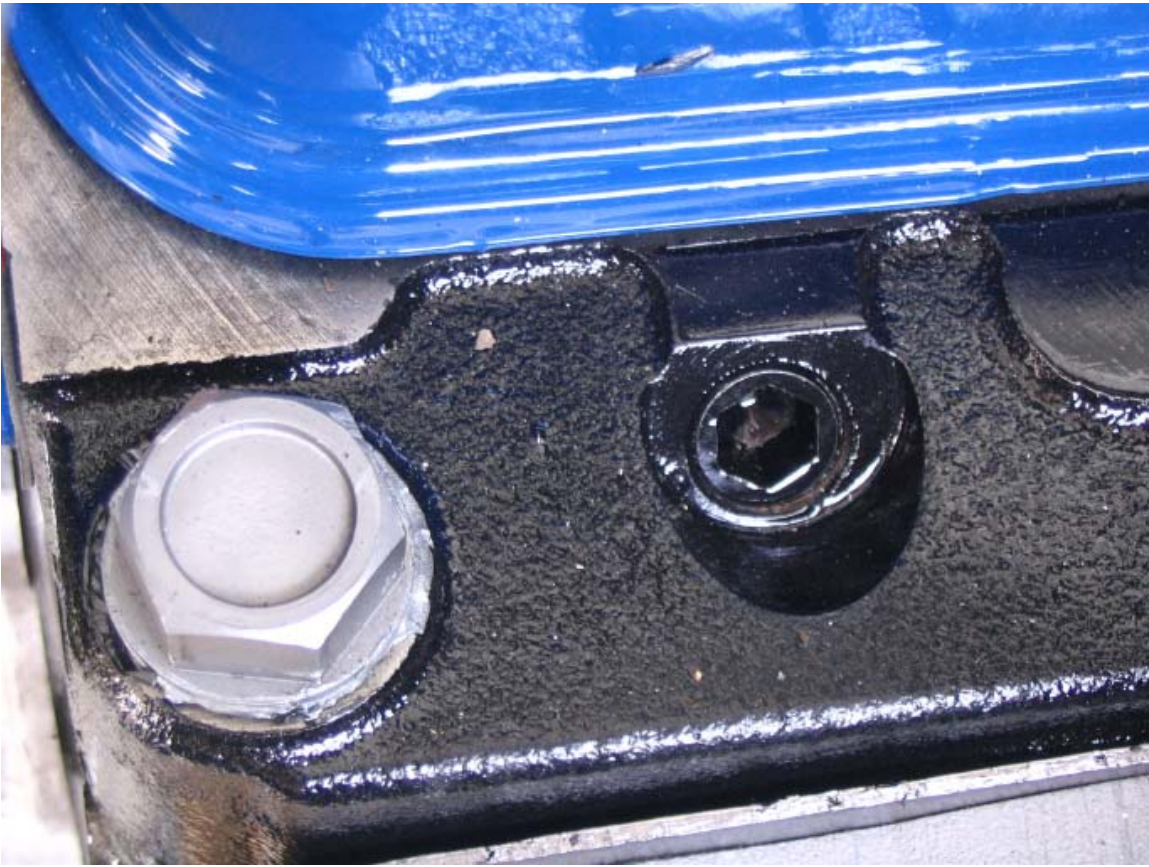
Figure 3. Allen head plugs on AI ports.
