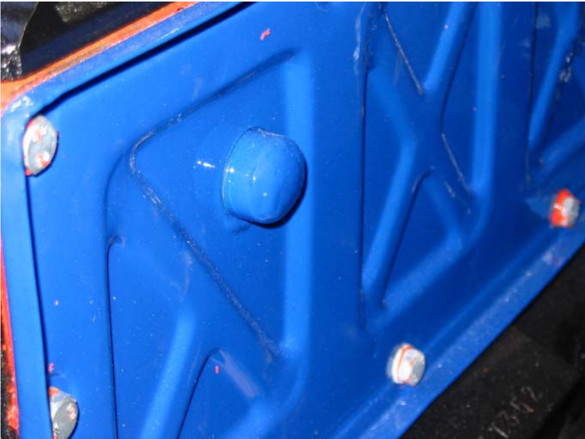
Figure 4. Plugged PCV port on 2F side cover.
