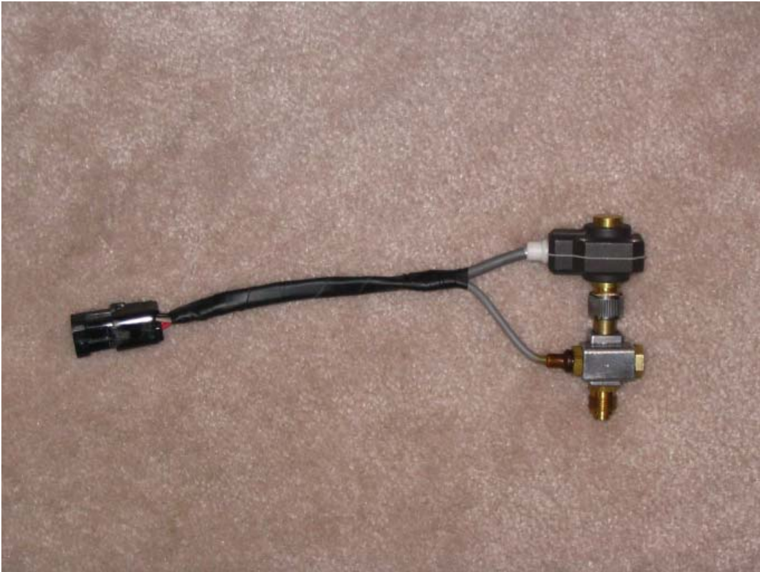
Figure 9. Piggyback vehicle speed sensors. Top is the VSS for the Autometer speedometer. Lower is the VSS for the ECU speed signal.
