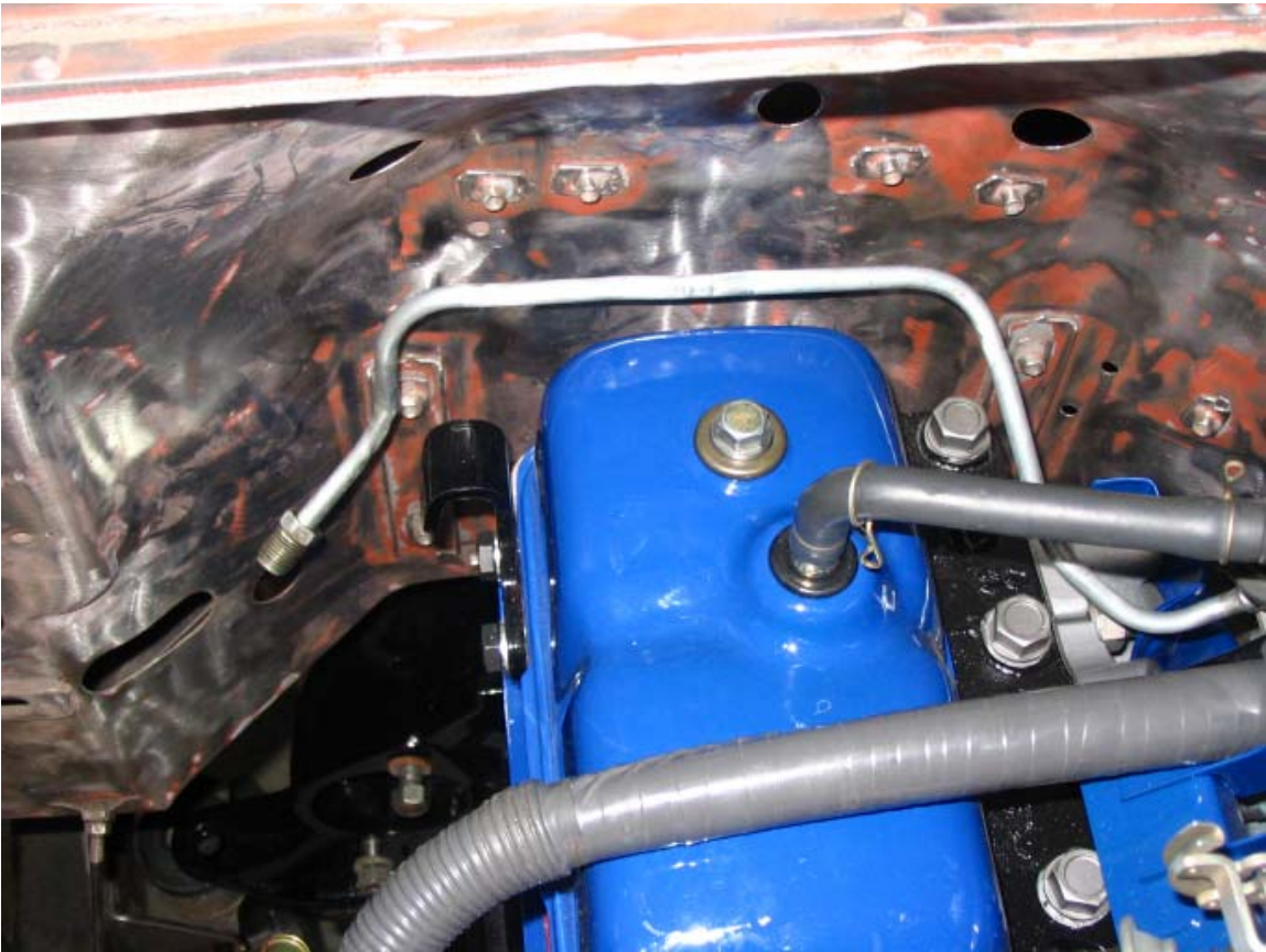
Figure 5. Rerouted fuel line behind head.
