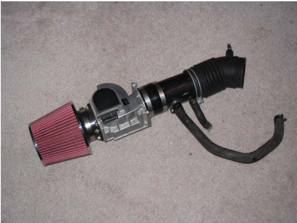
Figure 8. Intake showing steel pipe with double ports, one for breather, the second for ISC.
