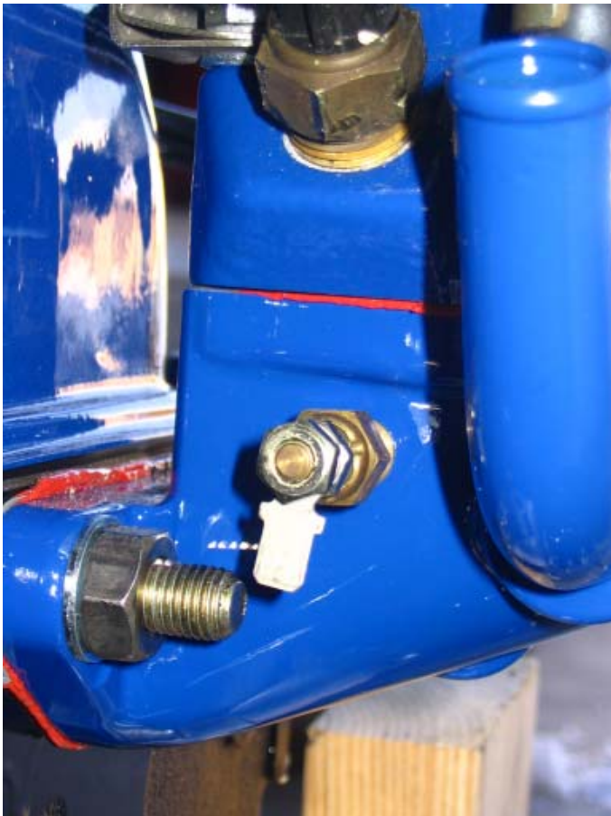
Figure 14. Location of aftermarket temperature sensor.
